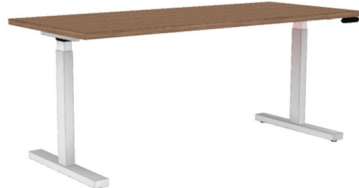
Agile (rectangle leg) Tubular foot, glide height range: 28.875"- 48.5"h Tubular foot, caster height range: 30.875"- 50.5"h Flat foot, glide height range: 28" - 47.625"h Flat foot, caster height range: 30" - 49.625"h
