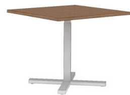
Applause square top X or H base Tubular foot, glide height range: 28.25" - 47.75"h Tubular foot, caster height range: 30.25" - 49.75"h Flat foot, glide height range: 27.25" - 46.75"h Flat foot, caster height range: 29.25" - 48.75"h
