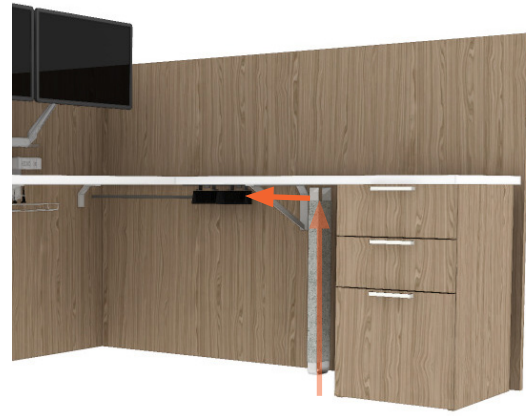
Floor core in middle of station
